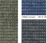
Flocked flooring 100cm x 25cm (2.5m² per box) Slip resistance Collection size Application EN-ISO 10874 Class 33 Impact sound EN ISO 717-2  $\Delta L_w = 19 \text{ dB}$ FN 14041 Reaction to fire EN 13501-1 B<sub>ff</sub>-s1, L, CS Slip resistance EN 13893  $\mu \ge 0.30$ Body voltage ISO 6356  $\leq 2.0 \text{ kV}$
